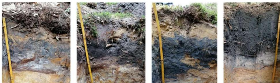
**Figure 5.** Fly ash Application as Soil Stabilization Agents in Various Dosages
