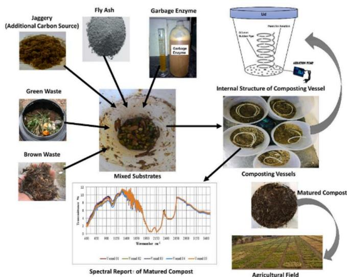
**Figure 6.** Scheme of Fly Ash Utilization with In-Vessel Composting System
